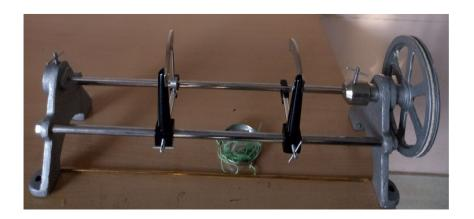
Apparatus consists of a wheel, moving on ball bearing provided with a chuck to hold the rod under test. The other end of the rod is clamped tightly to a bracket. The pointers and scales are graduated in single degree and can be clamped at any position. Apparatus is of horizontal bench pattern and is supplied complete with ribbon, hook, rods of steel and brass.
